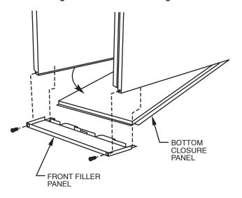
Fig. 25—Removing Bottom Closure Panel
